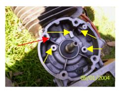
seal level and be concentric with crankshaft axis.
